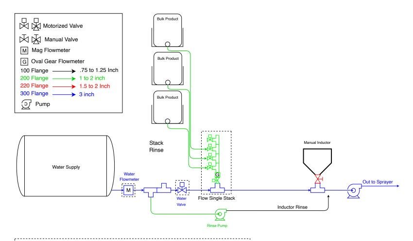
Mixmate three input Single Stack. All chemicals are measured with a gear type flowmeter. Up to one bulk chemicals will be measured simultaneously while using the inductor. Consult your dealer for variations to this configuration.
