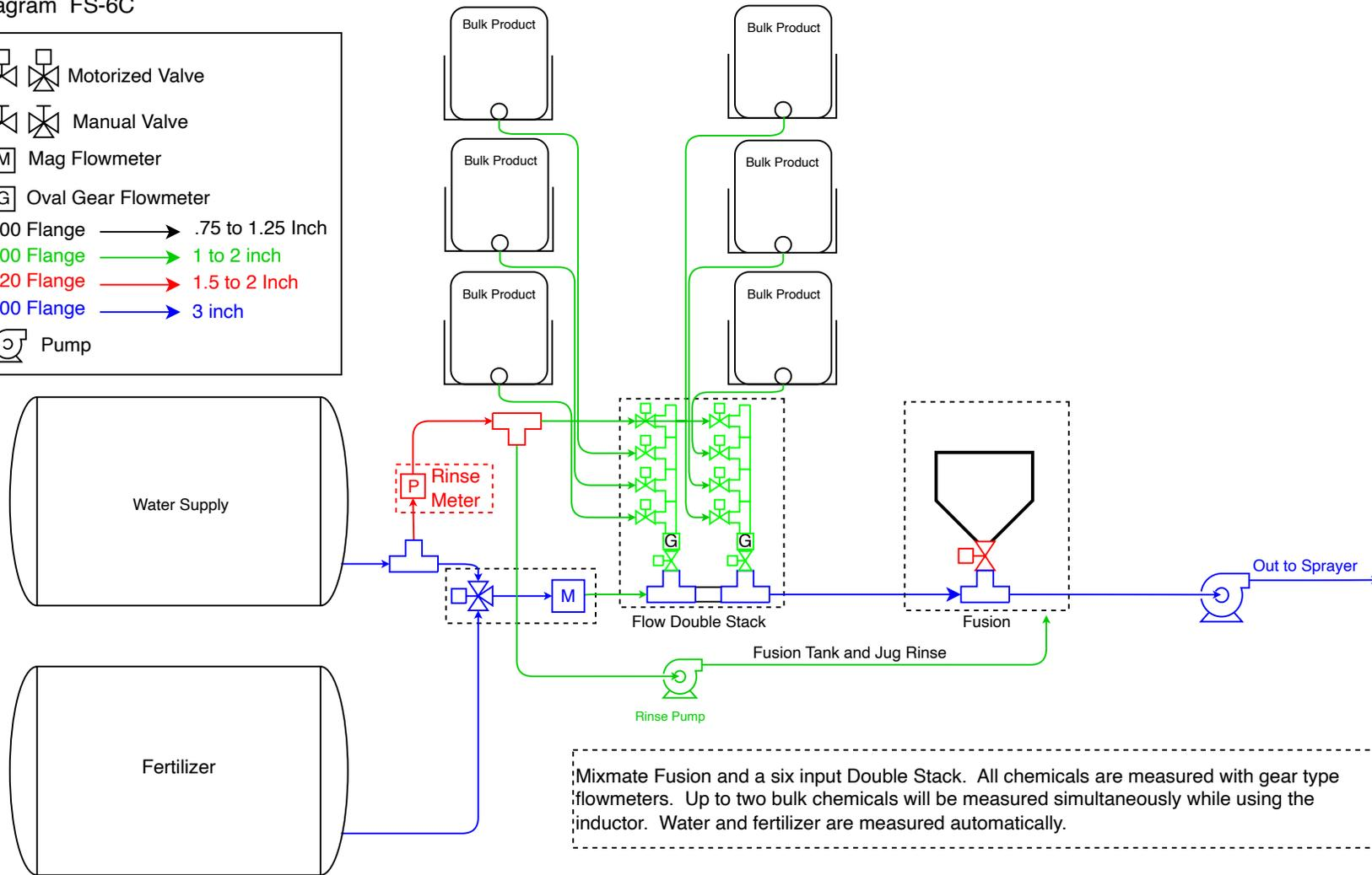
Mixmate Fusion and a six input Double Stack. All chemicals are measured with gear type flowmeters. Up to two bulk chemicals will be measured simultaneously while using the inductor. Water and fertilizer are measured automatically.
