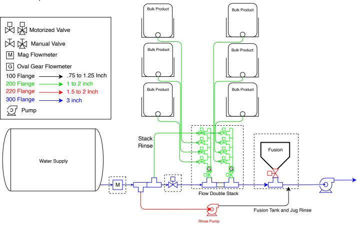
Mixmate Fusion and a six input Double Stack. All chemicals are measured with gear type flowmeters. Up to two bulk chemicals will be measured simultaneously while using the inductor. Water is measured automatically. Mixmate components in the dashed box.
